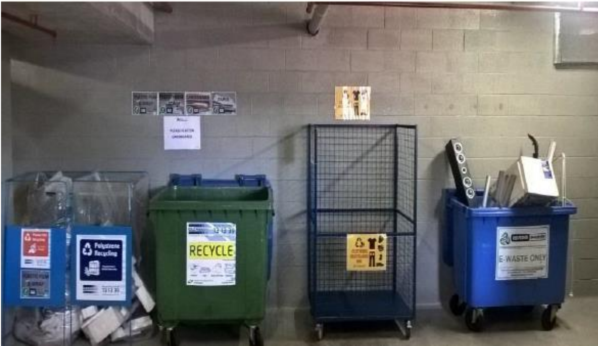
Figure 11 - With flexible space beyond the minimum allocated, it is easy to separate wastes and divert them to recycling (Source: State of NSW and NSW Environment Protection Authority 2019)
