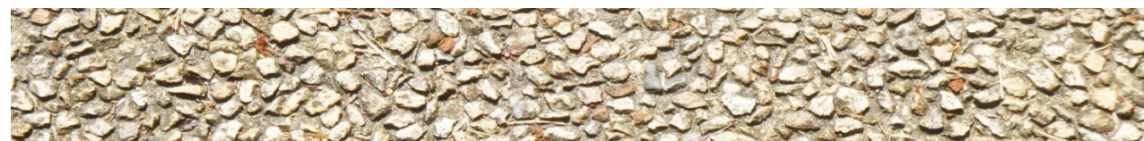
Example of coloured exposed aggregate concrete with rhyolite aggregate.
