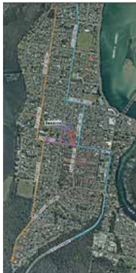
Swansea evacuation routes, developed as part of a Swansea Flood Study (Umwelt 2016)
