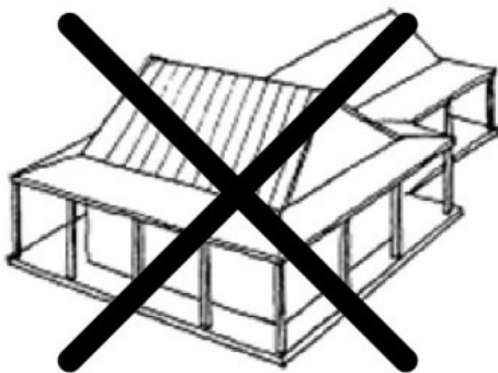
Minor wing extension to rear, with a wrapped verandah around the house. This form of verandah is not appropriate for Catherine Hill Bay
