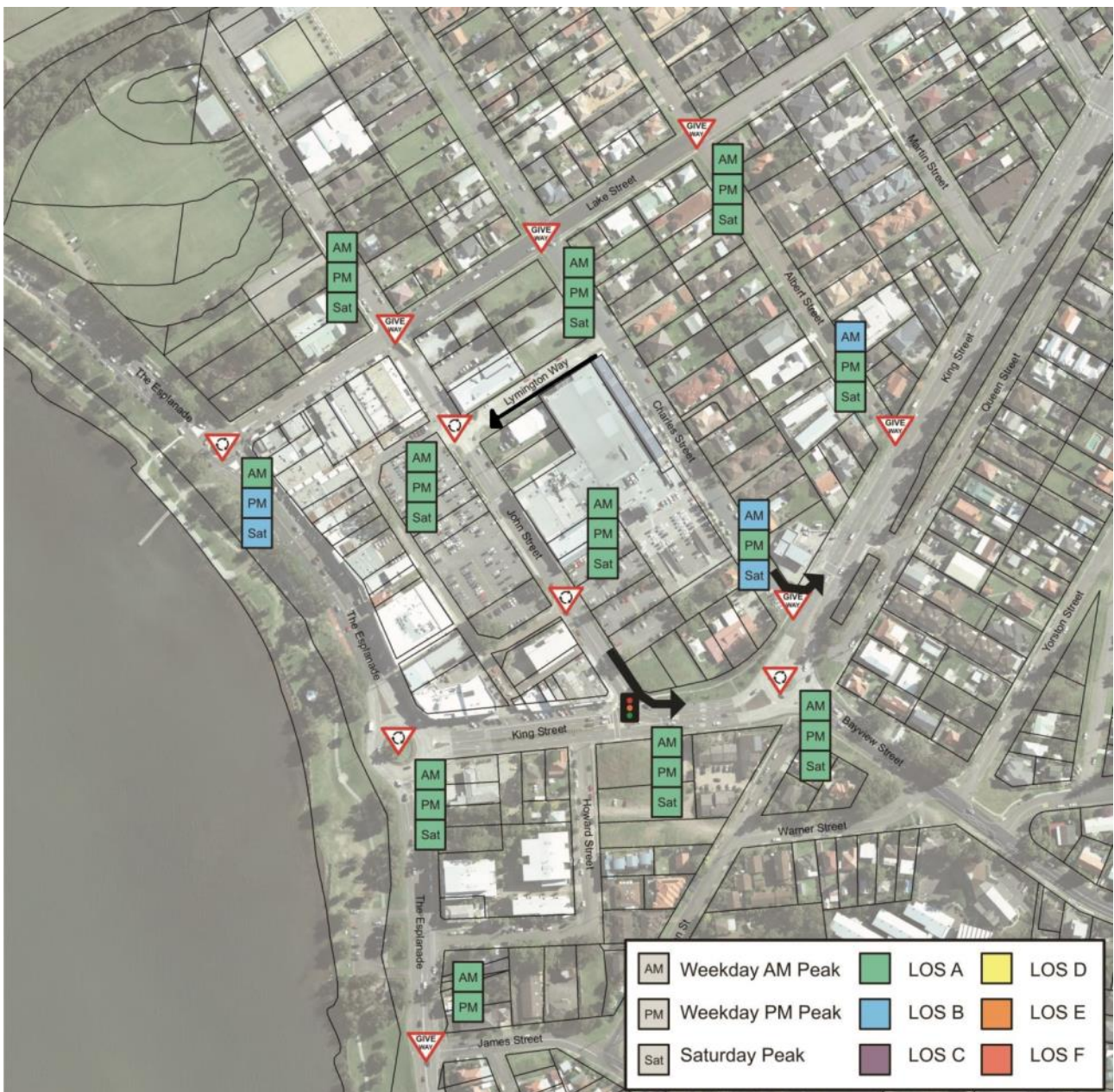
Figure 30 - Existing intersection operations with left turn only movements at John and Charles Streets
