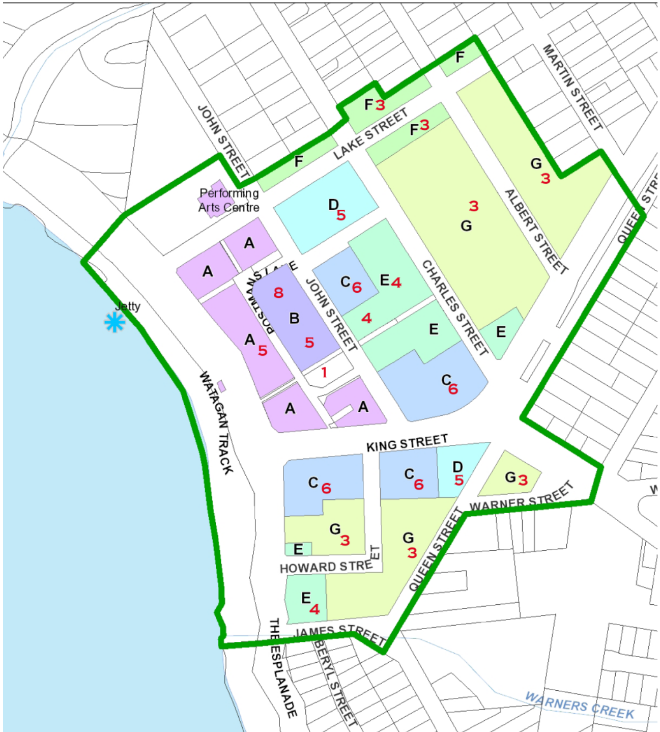
Figure 76 - Proposed building types with their maximum heights in storeys above ground (shown in red).
